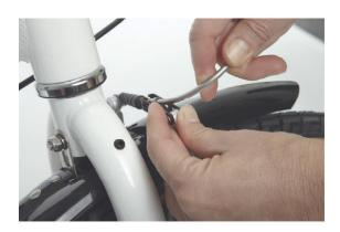
2. Disconnect the rubber contact from the motor
