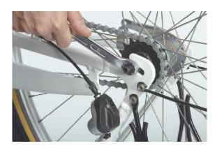
5. Loosen the hub bolts6. Push the wheel forward and release it from the chain
