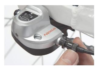
4. Turn the adjusting cable so that the yellow mark is in the middle again and tighten the nut
