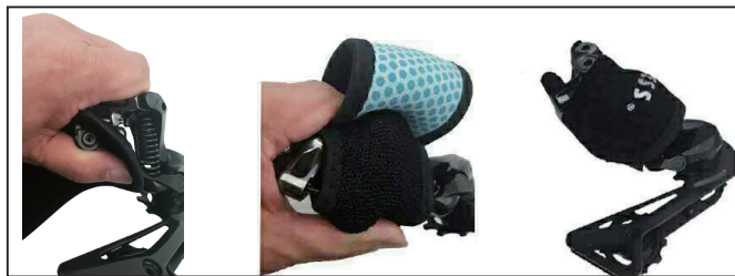
3 As shown in the illustration: For disassembling easily and make more space between the cage and the body of rear derailleur. Please use velcro tie or nylon cable tie etc. to fix the four bar linkage and keep the position.
