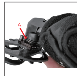
7 A: First, fix RIDEA RD6 rear derailleur cage into the body. Please do not press to the end, and reserve the space for rotating.
