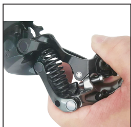
2 First of all, please expand the four bar linkage of rear derailleur cage to maximum position.
