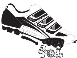
Insert front part of cleat into pedal and then snap the rear part.
