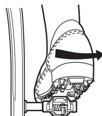
Turn heel in direction out of bike and release the cleat from pedal.
