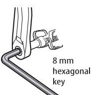
Before the assembling of pedals, lubricate threads by vaseline to protect them against corrosion.
